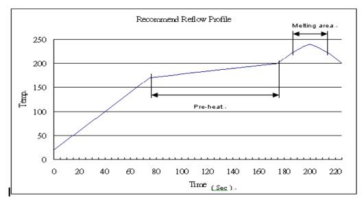
Fig. 8 IR Reflow Profile
