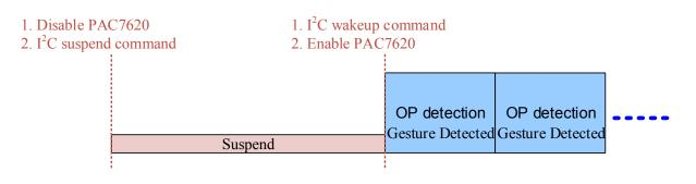
Figure 12. Suspend State (SUS state) Diagram
