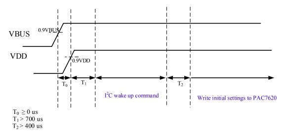
Figure 5. PAJ7620U2 Power-On Timing Diagram
