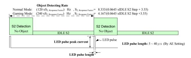
Figure 11. Standby 2 State (S2 state) Diagram
