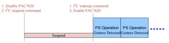
Figure 15. Suspend State (SUS state) Diagram
