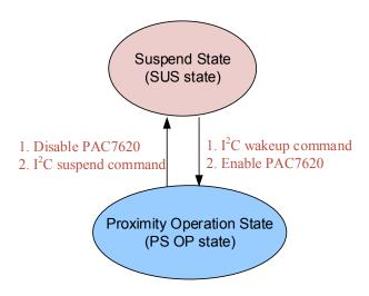
Figure 16. State Machine of Gesture Detection
